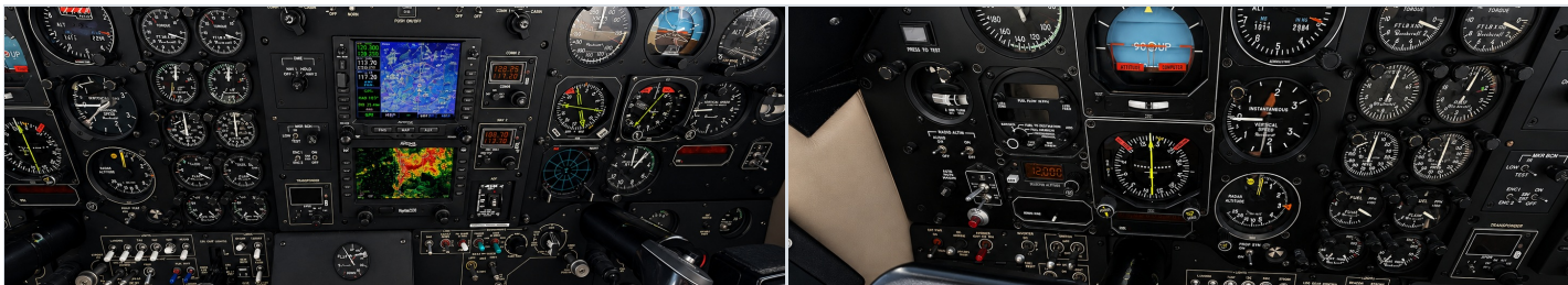
INSTRUMENT PANEL — AVIDYNE IFD-540 & PILOT STATION
