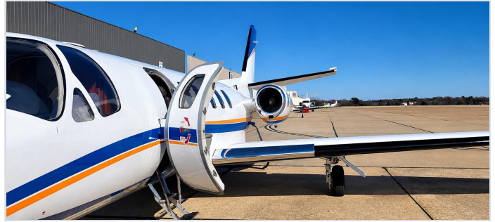
AIRSTAIR ENTRY DOOR
